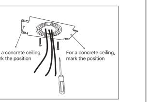
2. Fix the mounting plate securely to the junction box again and secure it by adding two wood screws to the outer holes.
