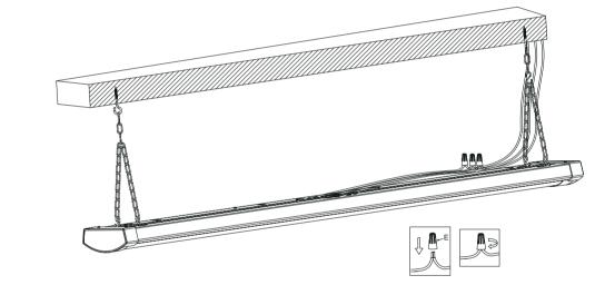
5. Connect to the driver according the color of wires with wiring cap.
