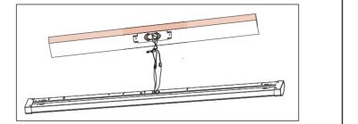
5. Hang the lamp on the prepared wood screws using the church key holes on both upper sides of the lamp. It may be required to adjust the tightness of the screws. Make sure the screws hold the lamp securely on the narrowed side of the church key holes.
