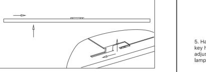
1. Directly screw four wood screws into the installing surface according to the distance of each church key hole. Do not screw them too tightly. For a concrete ceiling, it is required to drill two mounting holes first and then use the screw anchors and screws.
