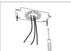
3. Connect the quick coupling with the mains supply using the wire nuts. Also use a wire nut to connect the ground wire connector with the ground connection.
