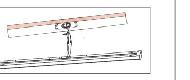
6. Hang the lamp onto the holding plate and ensure it is locked
