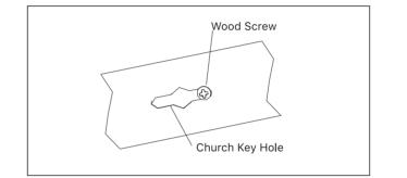
6. Mount the fifth wood screw next to the side of opposite pushing direction to lock the lamp. For a concrete ceiling, mark the position for a suitable hole. Take off the lamp. Drill the hole on the marked position and strike one screw anchor inside. Hang the lamp as described in step 5 and then screw the third screw into the prepared screw anchor to securely lock the position of the
