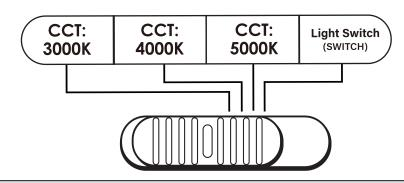
**NOTICE:** The toggle switch is located on the back of the fixture.
