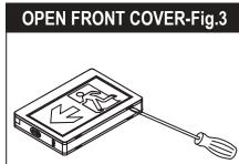
Open front cover with blade screwdriver
