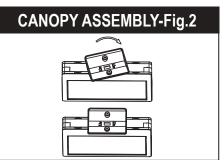
Insert canopy into housing at 20 degree angle and twist. Quick snap is now firmly locked.
