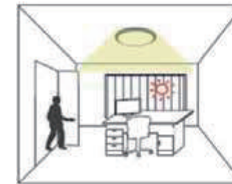
The fixture will turn on when motion is detected, regardless of the presence of natural light.
