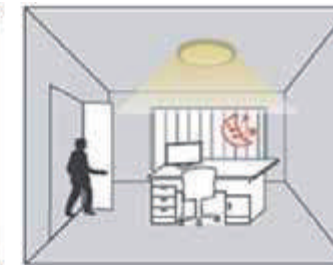
The fixture will turn on when motion is detected, regardless of the presence of natural light.
