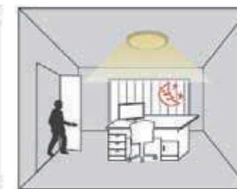
When no natural light is detected, the fixture will turn on when someone enters the room.
