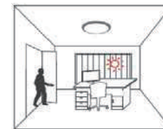
When the room is illuminated with natural light, the fixture will not turn on when someone enters the room.
