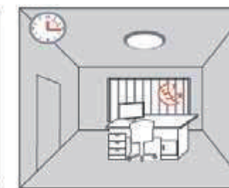
The fixture will remain in standby mode when no motion is detected.
