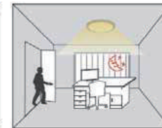
When no natural light is detected, the fixture will turn on when someone enters the room.
