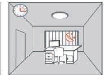
The fixture will remain in standby mode when no motion is detected.
