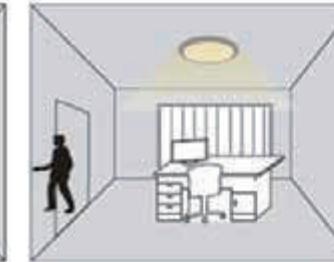
The fixture will remain on for 30seconds, or until no motion is detected.
