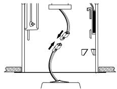
Insert the torsion springs into the fixture housing brackets. When installing the product into a 5 in. recessed housing, the torsion spring must be moved. Unscrew the torsion spring from the 6 in. position and move to the 5 in. position.
