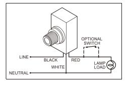
5) Switch the power on to the circuit. The controlled load should turn on and if it is daylight, turn off within a few minutes.
