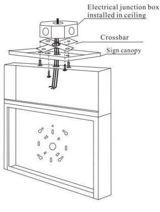
3. Make the proper supply lead connections.
