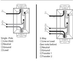
IMPORTANT Please note that for 3 -way application, there have a power cord from the original switch be a different color (Black) or marked Common. Finding this power cord from both the dimmer's junction box and 3 -way junction box and marking as common (live or load).
