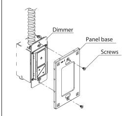
• Put the panel and panel base together, press gently to make sure it is be installed firmly.
