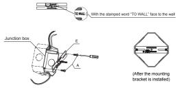
② Connect ground wire with terminal ① with ground wire in the junction box, screw on the wire nut ⑥ to secure.
