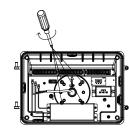
6.Lock the bottom shell on the mounting seat with screws,Connect the L, N and G wires to the power supply.
