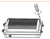
2.Use a screwdriver to remove the screws on both sides and remove the upper cover of the fixture.
